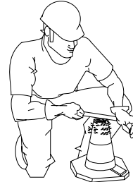
Figure Q. Slump Test (Removing Excess Concrete)
